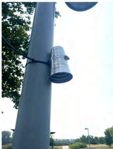
Sorbent Tube System with pole mount installation
